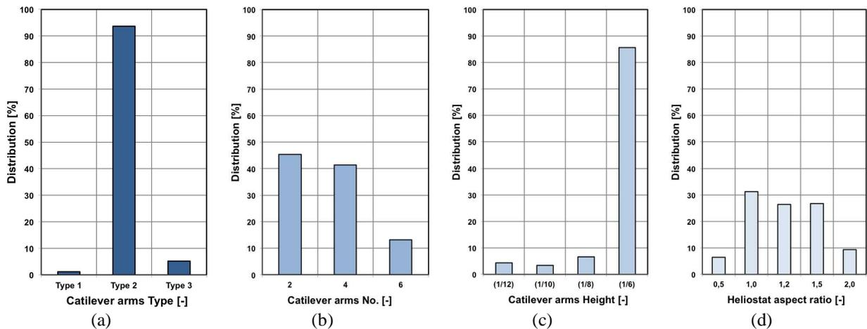
FIGURE 12. Distribution of the incremental changed parameter- Operational mode: (a) Cantilever arms type, (b) Number of cantilever arms, (c) Cantilever arm height, (d) Heliostat aspect ratio
