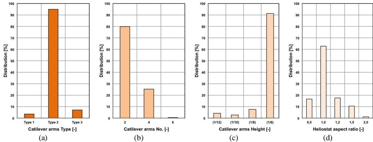
**FIGURE 13.** Distribution of the incremental changed parameter - Survival mode: (a) Cantilever arms type, (b) Number of cantilever arms, (c) Cantilever arm height, (d) Heliostat aspect ratio
