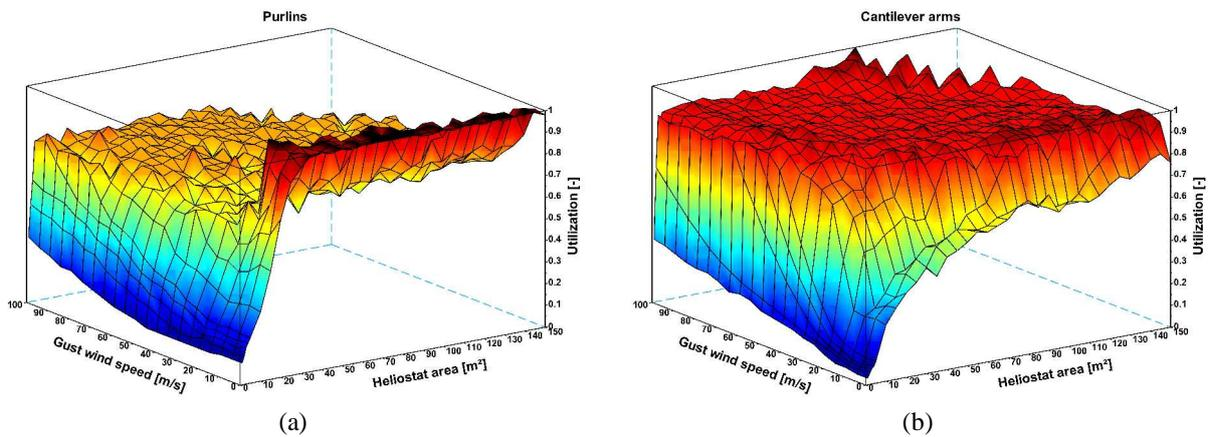
**FIGURE 5.** (a) Purlin utilization: mean = 67.1%; (b) Cantilever arm utilization: mean = 77.7%.
