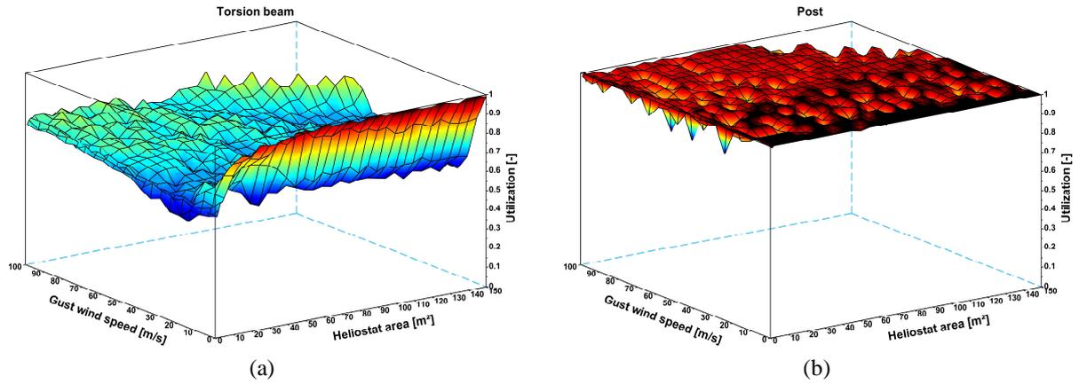
FIGURE 6. (a) Torsion beam utilization: mean = 71.4%; (b) Post utilization: mean = 98.4%
