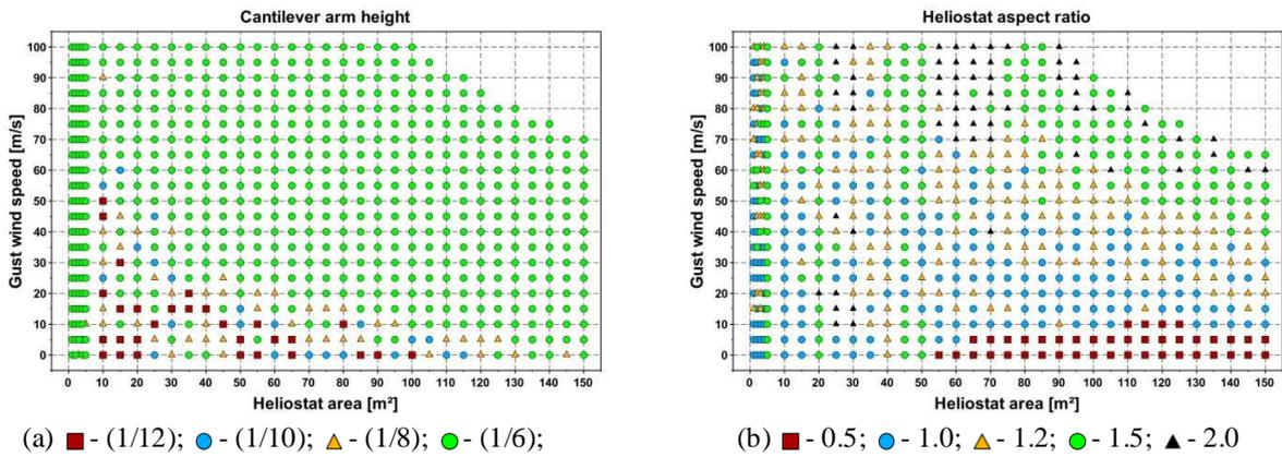
**FIGURE 4.** (a) Cantilever arm height as a function of the half height of the heliostat; (b) Heliostat aspect ratio.
