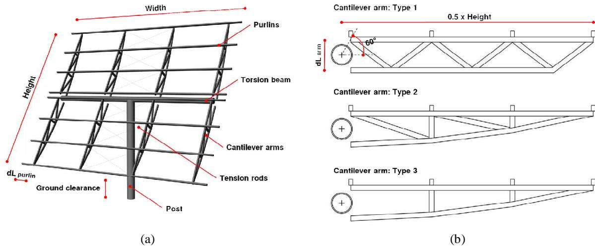
**FIGURE 1.** (a) Structural members of the heliostat; (b) Three different cantilever arms.
