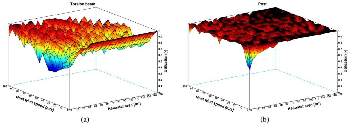
FIGURE 11. (a) Torsion beam utilization: mean = 84.5%; (b) Post utilization: mean = 97.9%
