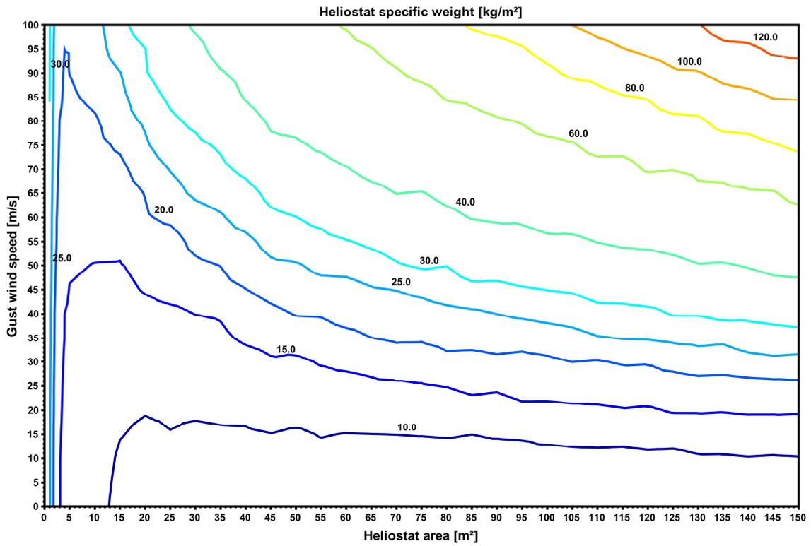
FIGURE 7. Specific weight of the heliostat in [kg/m²] as a function of gust wind speed [m/s] and heliostat area [m²]
