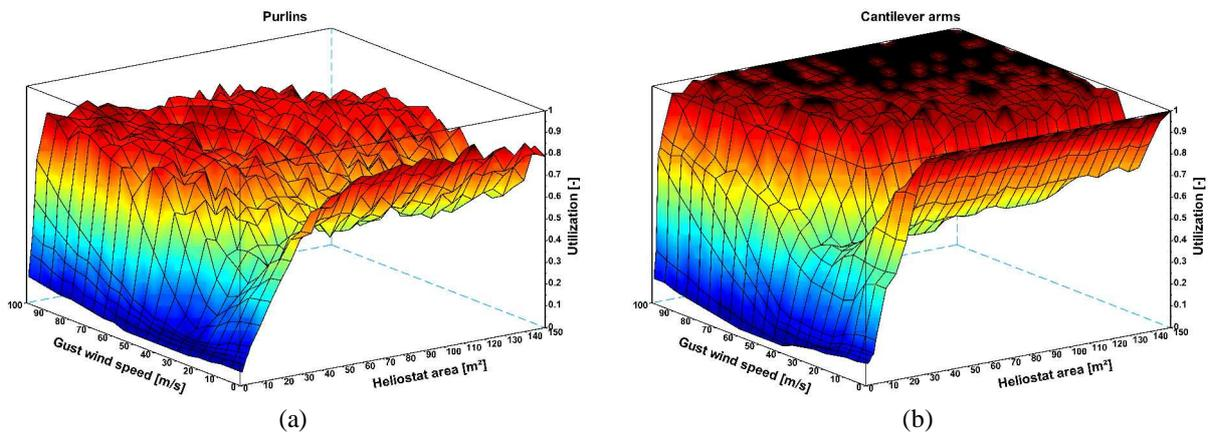
FIGURE 10. Purlin utilization: 62.4%; (b) Cantilever arm utilization: 79.3%.
