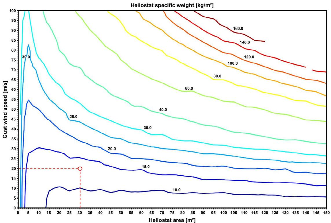
FIGURE 2. Specific weight of the heliostat [ $\text{kg}/\text{m}^2$ ] as a function of gust wind speed [ $\text{m}/\text{s}$ ] and heliostat area [ $\text{m}^2$ ]
