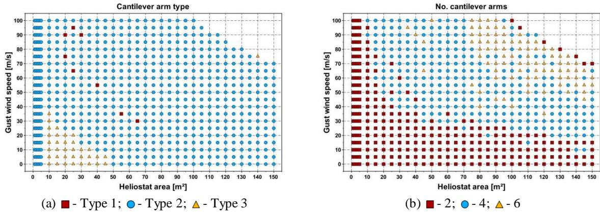
**FIGURE 3.** (a) Cantilever arm type; (b) Number of arms.
