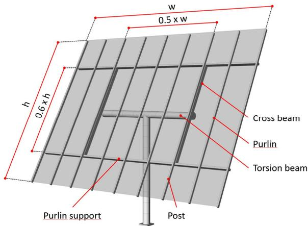
Fig. 3. Tracker parameterization
