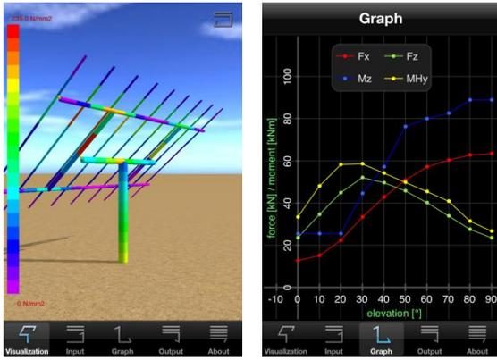
Fig. 2. FEM model (left), forces and moments acting on the tracker (right)
